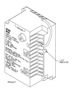
A steady L.E.D. indicator indicates normal operation.
